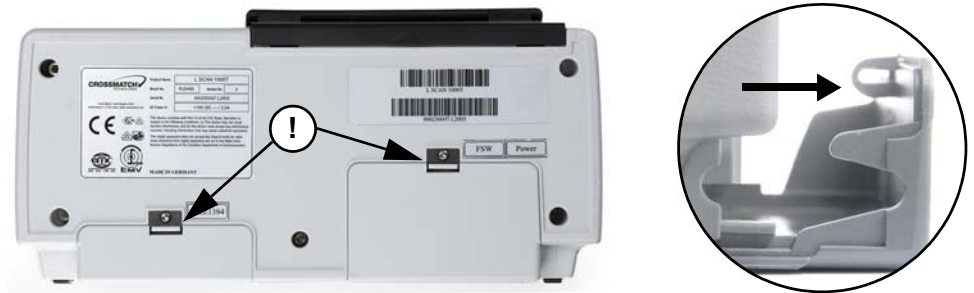
Figure 3.3 Removing the connector tray covers
