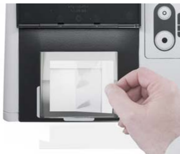
Figure 5.10 Place and press cleaner sheet to silicone pad
