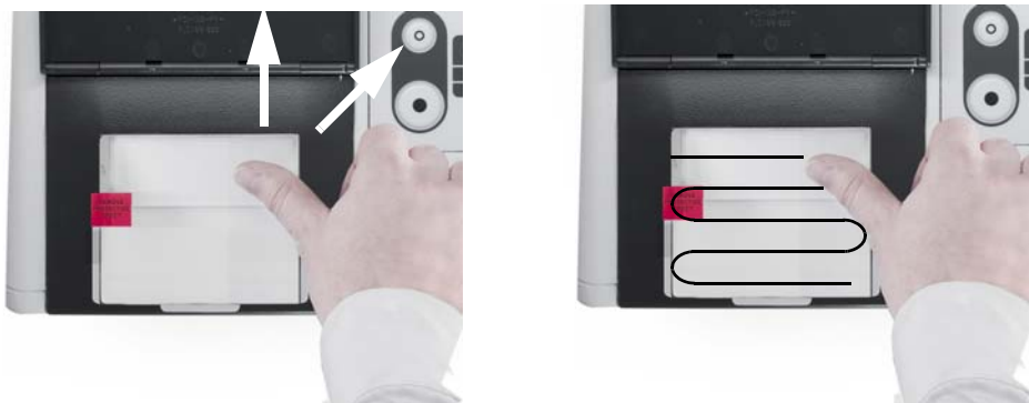
Figure 5.7 Wiping bubbles from silicone pad
