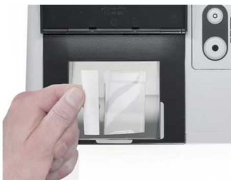
Figure 5.11 Lift cleaner sheet off silicone pad
