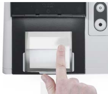
Figure 5.10 Place and press cleaner sheet to silicone pad
