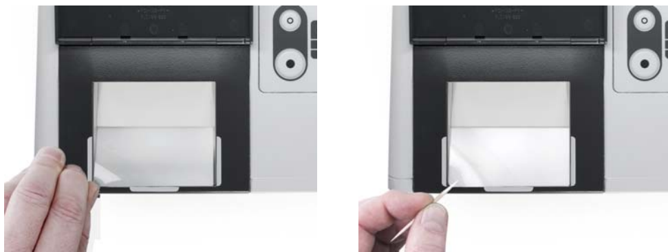
Figure 5.4 Prying up a corner of the silicone pad
