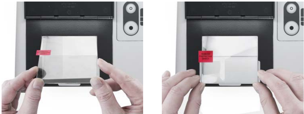
Figure 5.6 Adjust and lowering the silicone pad
