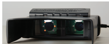
I SCAN 2 captures iris images in less than ten seconds and weighs just over one pound
