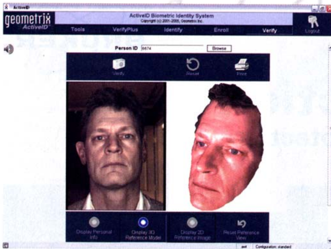
A verification side-by-side view featuring a 2D verification image next to a 3D enrollment model
